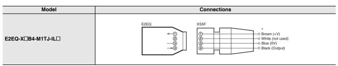
\* If the XS5W-D42---81-F Connector which has a socket and plug on the cable ends is connected to the Sensor, this part will be a plug.
