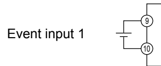
Input with voltage (PNP)
