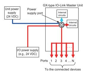
**Note** Even if the Unit power supply is not supplied, if you supply the I/O power supply, the I/O power supply is supplied to the connected devices from the ports.
