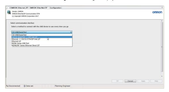
There are the following interface types according to the different connection path.
