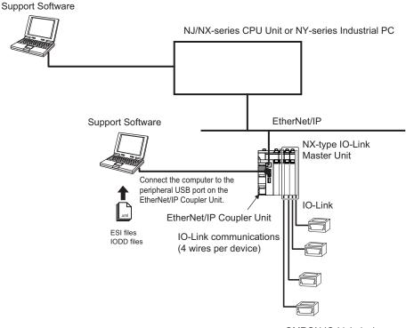
OMRON IO-Link devices or IO-Link devices from other companies<sup>\*1</sup>
