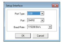
2 Set the **Port Type**, **Port**, and **Baud Rate** to suitable values and then click the **OK** Button to connect to the CJ2-series PLC. If the connection is successful, the **Browse Network** Dialog Box is displayed.
