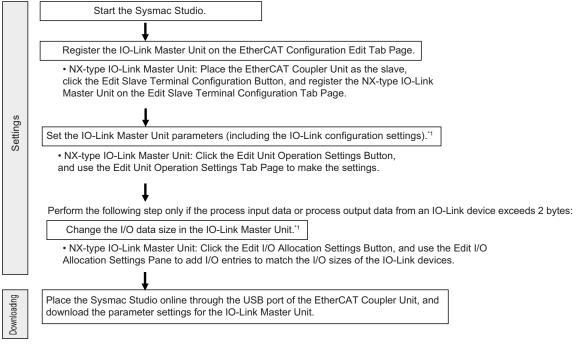
Note: Use the software application from the other company to perform PDO allocations for EtherCAT communications and to program the controller.
