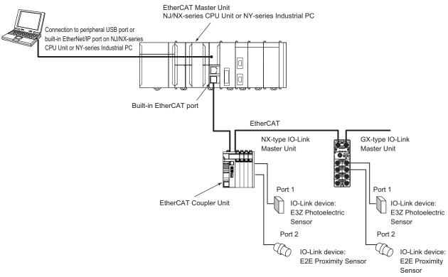
For the above system configuration, use CX-ConfiguratorFDT to create a network configuration as shown below.
