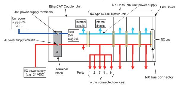
**Note** Even if the Unit power supply is not supplied, if you supply the I/O power supply, the I/O power supply is supplied to the connected devices from the ports.
