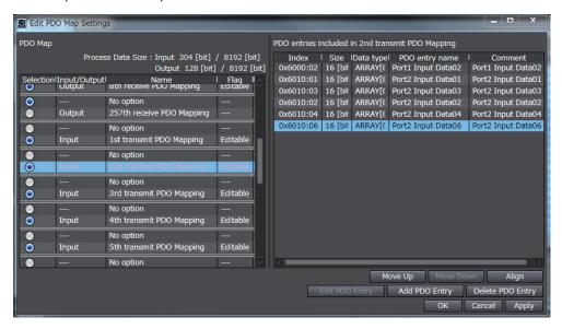
To save the I/O data size for unused ports, clear the selections of the PDO mappings for the unused ports in the PDO mapping list.
