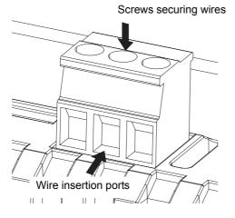
**3** Insert the wires and tighten the screws.
