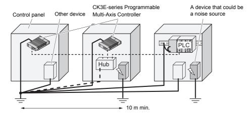
(b) Connecting devices and noise sources to a common earth electrode
