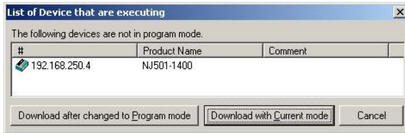
Fig. 7-20 Download with Current Mode
